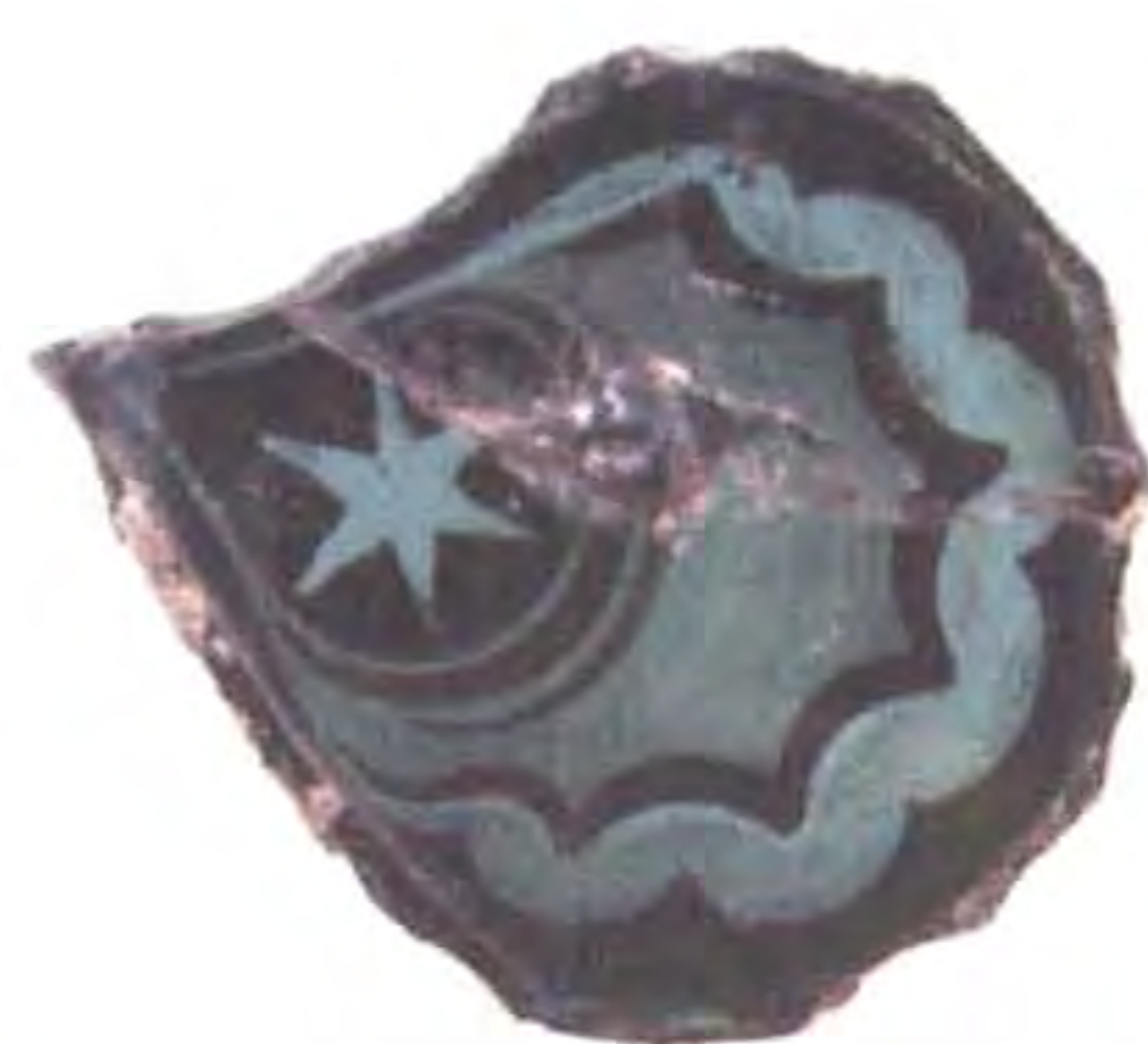
Figure 31: A piece of cloud with a defect caused during the blowing of the glass
