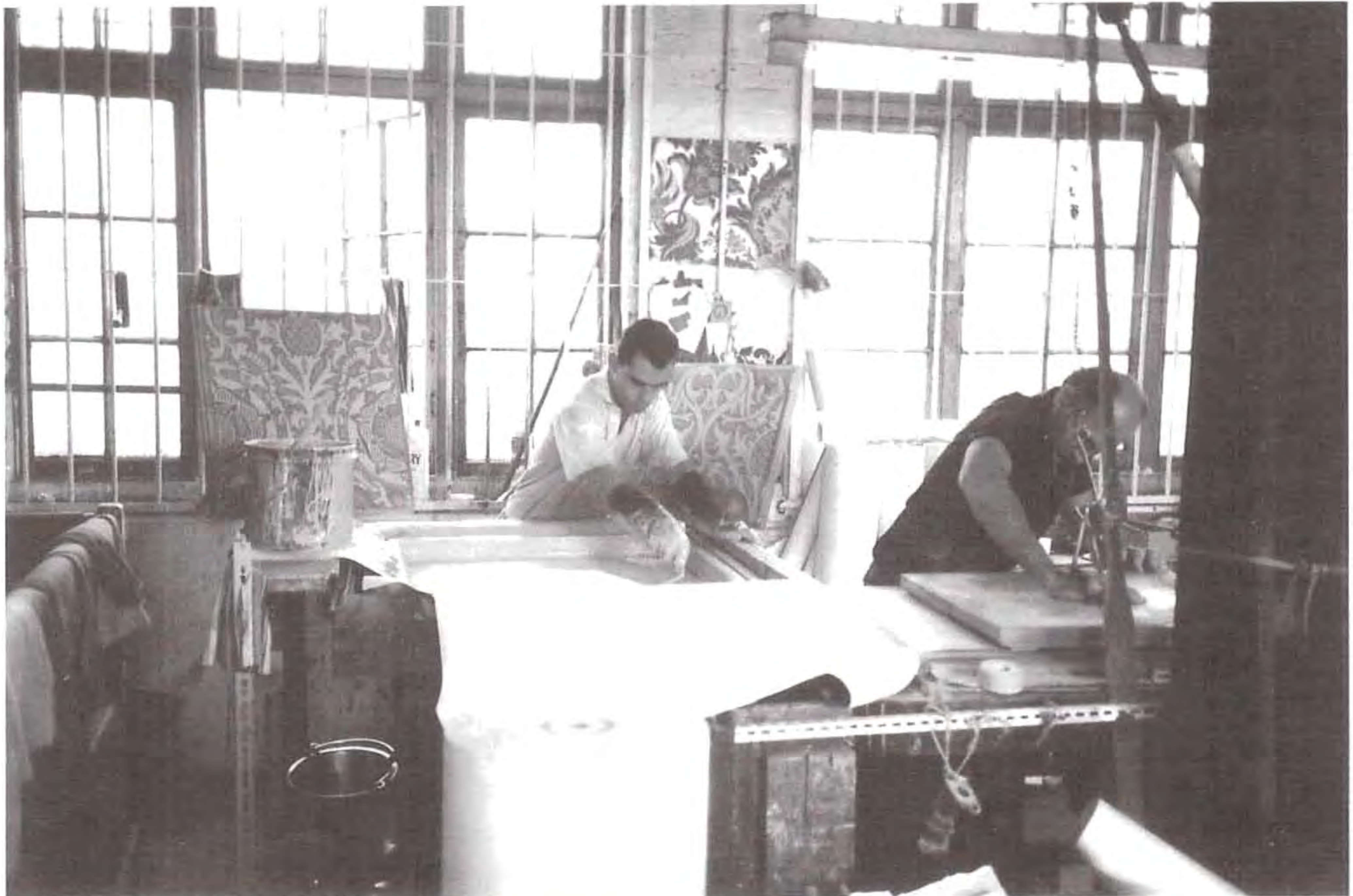
Figure 27: The interior of the former workshop of Cole and Son, Islington, in 1991 during the blocking of the wallpaper for the Prime Minister's room. To the left, ink is prepared before being applied to the blocks (shown behind). To the right, a block is applied to part of a roll of paper using suspended callipers and then pressed down by hand
