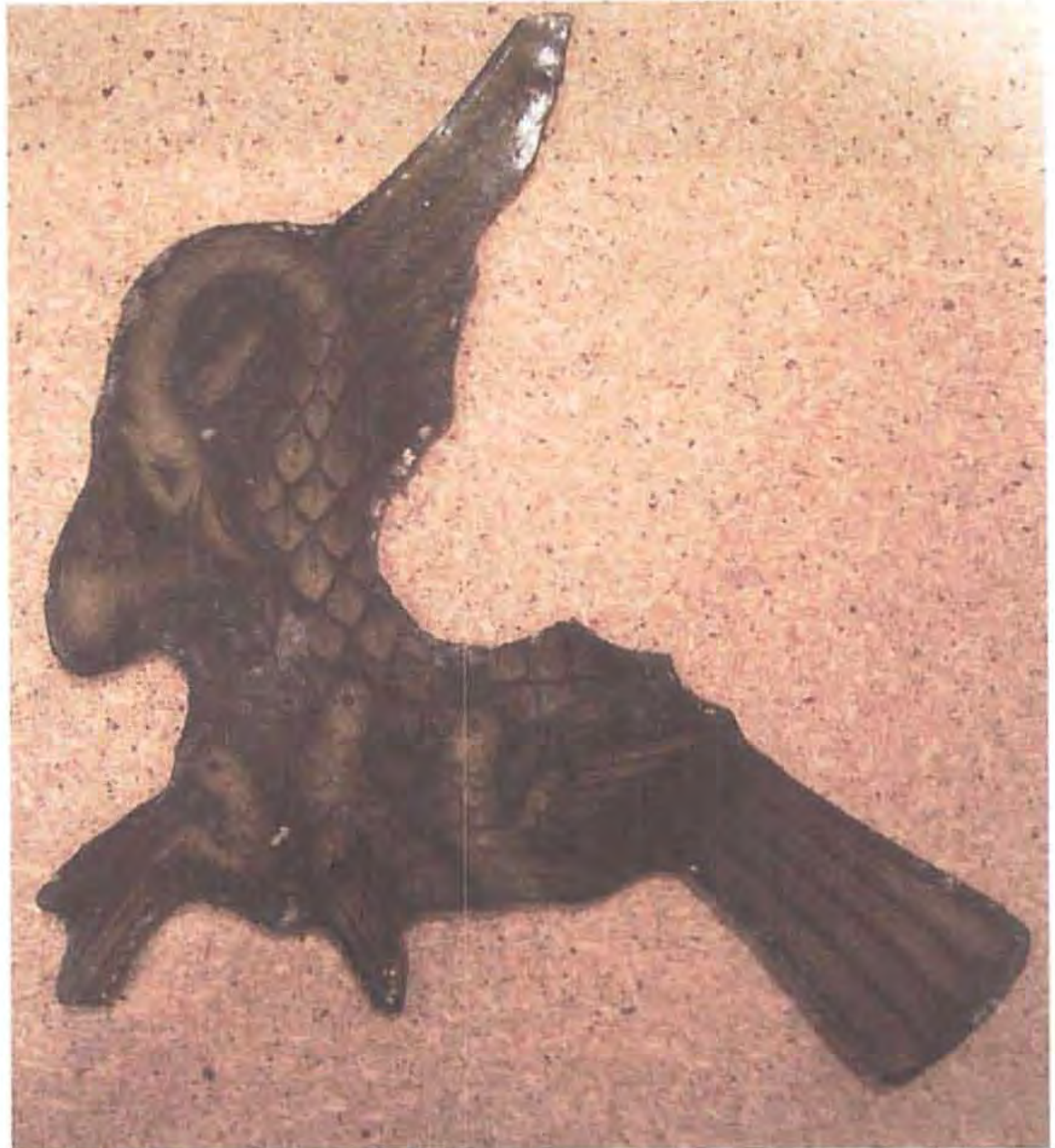
Figure 38: A complex piece of glass cutting by grozing
