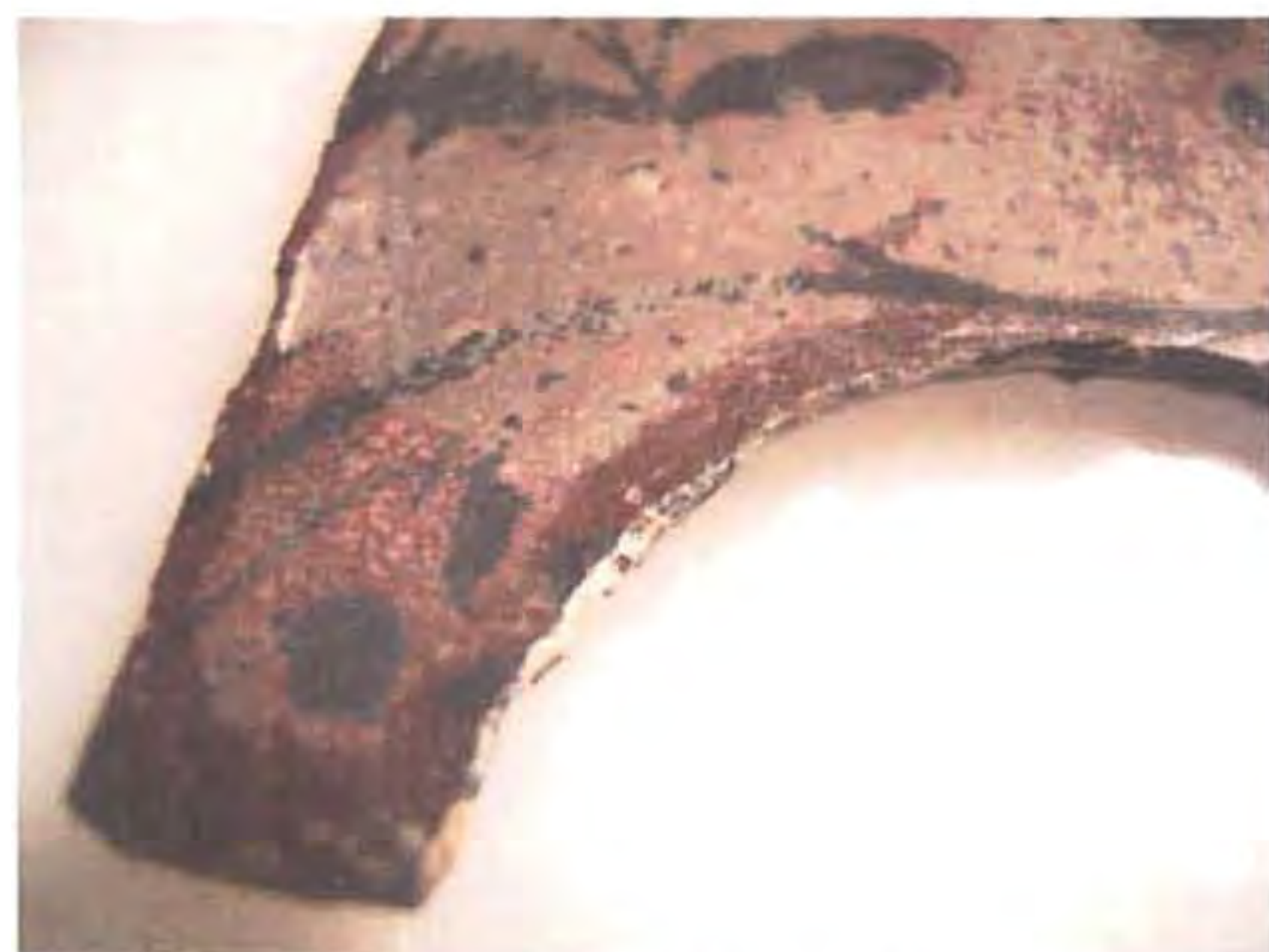
Figure 41: Under-fired glass showing paint not fully adhered
