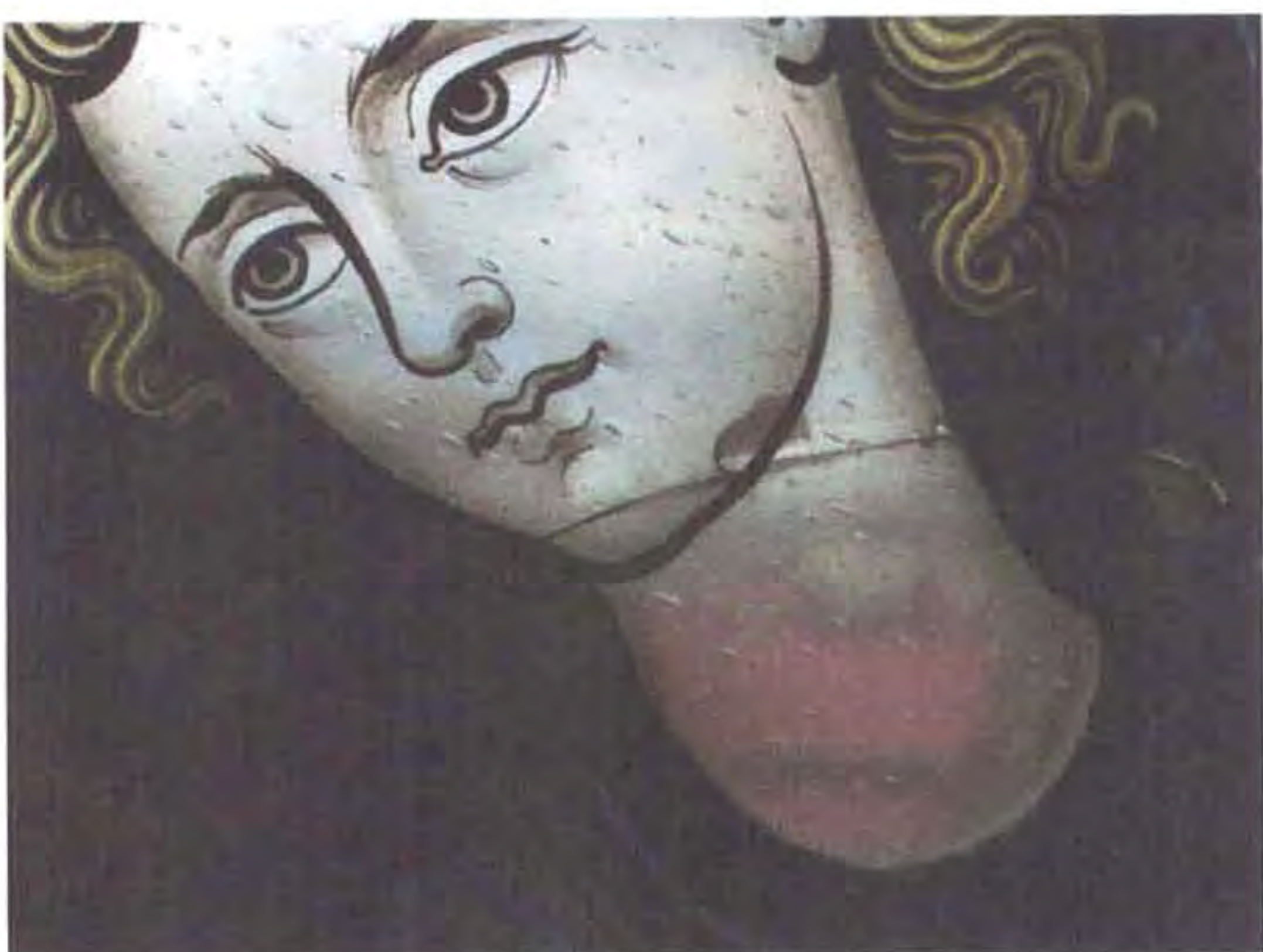
Figure 32: A large gas bubble that caused the glass subsequently to crack
