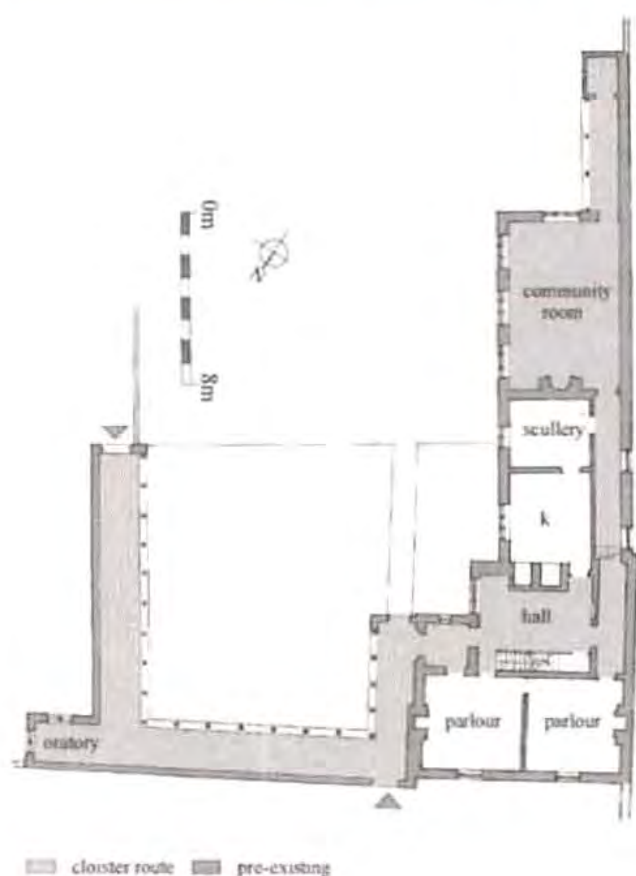
Figure 48: Pugin's unconventional plan of the Cheadle convent, showing how the whole of the building is arranged around a long corridor Brittain-Catlin 2006, p 365 fig 14.
